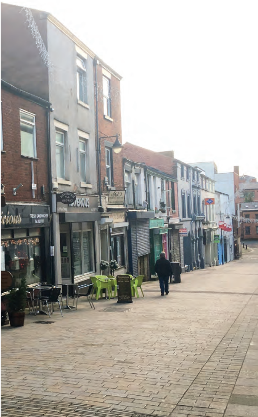
Cannon St, Preston Pedestrian priority design: stone pavements, and space for businesses' spill-out. Signage has been located along the building line to avoid clutter.
